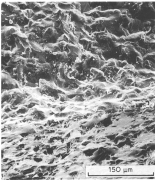
Figure 8 SEM of porcelain (hipped) fracture surface.
