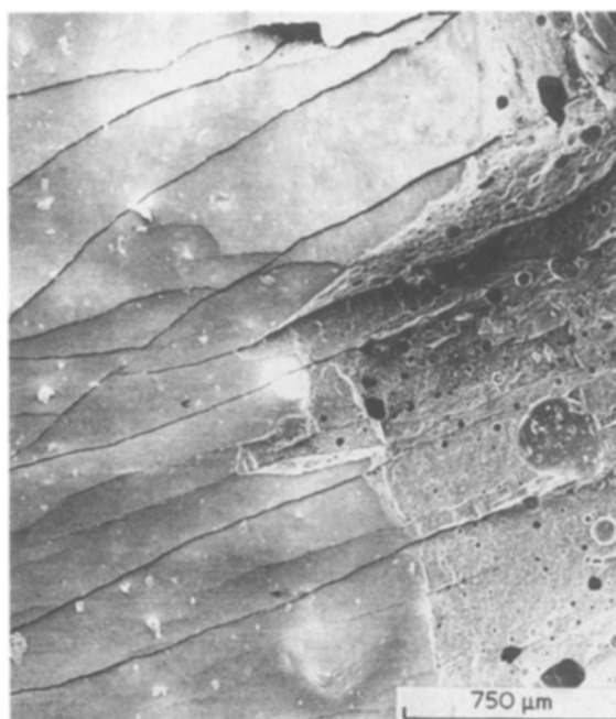
Figure 3 SEM of Au alloy bond (normal) fracture surface.
