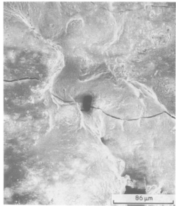
Figure 6 SEM of Au alloy bond (hipped) fracture surface.
